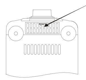
RESET button hole (Press the button inside with a non-metal stick)
